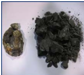
Alloy and Slag from the first smelting test of Big Daddy ore
